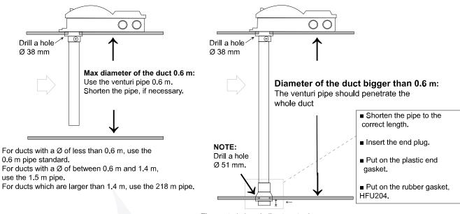
The venturi pipe shall not protrude more than max 30 mm through the duct wall.
