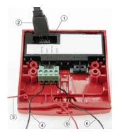
The FC420CP-I has a factory set (invalid) address of 255. The FC420CP-I is field programmed with the address prior to installation using an FireClass address programming tool. The associated ancillary programming lead plugs into the programming port. Ensure that the pins of the ancillary programming lead are inserted completely into the lower row of the programming port for effective communication with the address programming tool.
