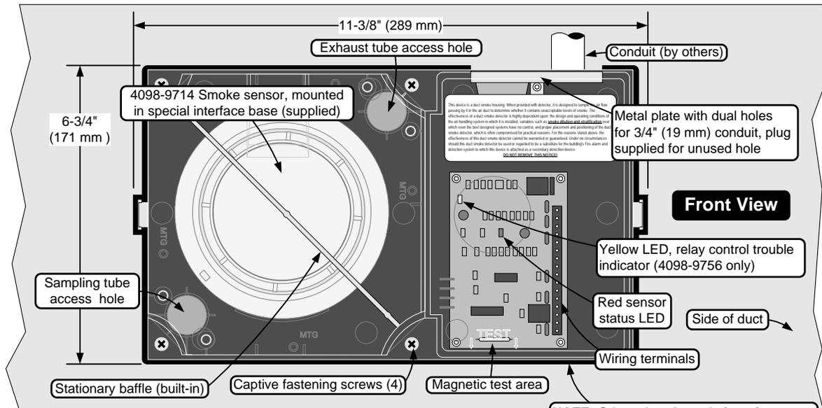
**NOTE:** Orientation shown is for reference only, refer to General Location Notes and End View illustration below for alternate mounting reference.
