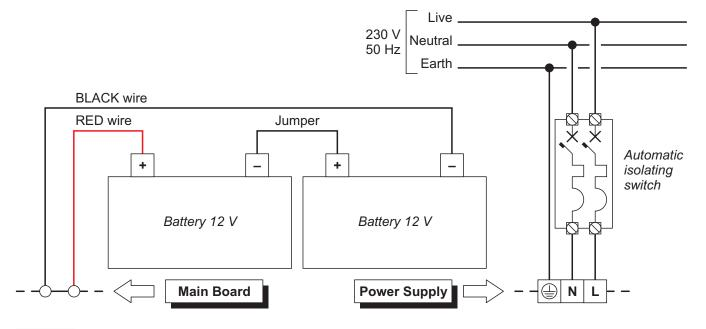
Figure 11 Wiring diagram for the power supply.
