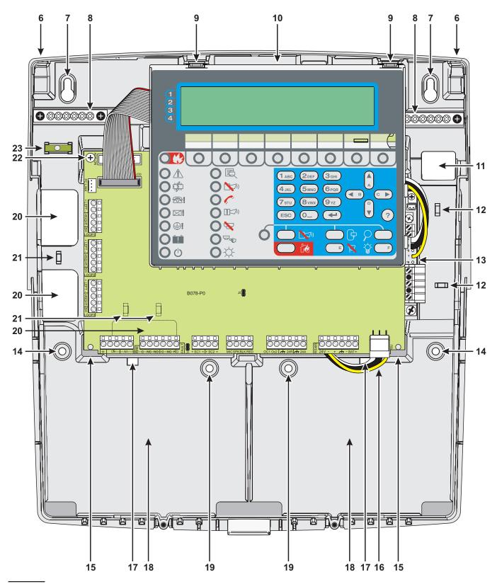
Figure 2 FC501 Parts: external view.
