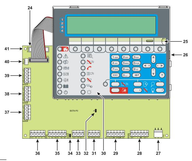
Figure 3 Main module Parts.
