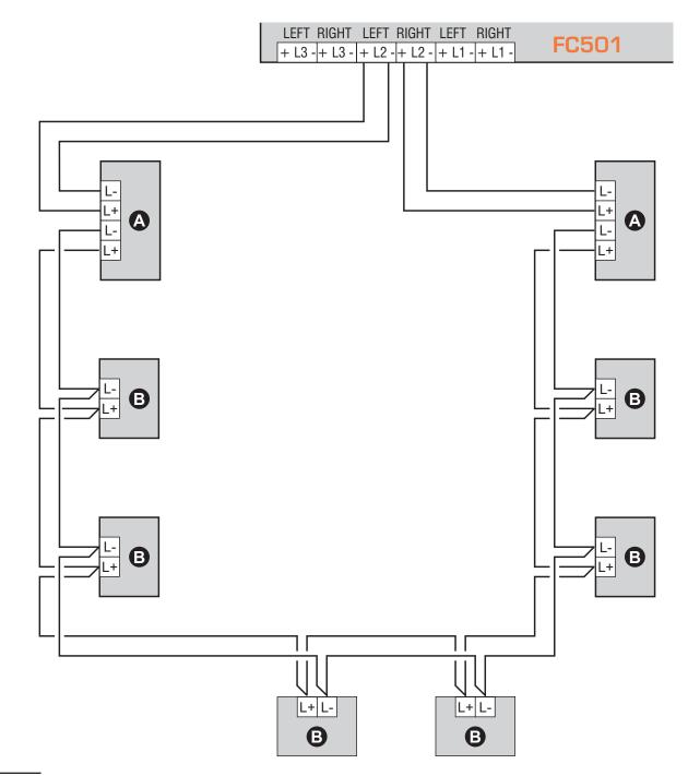
**Figure 7** Wiring diagram of a 4-wire connection: **a**) Isolators; **b**) Compatible analogue devices (Fire detector, Input modules, Output modules, Manual callpoints).
