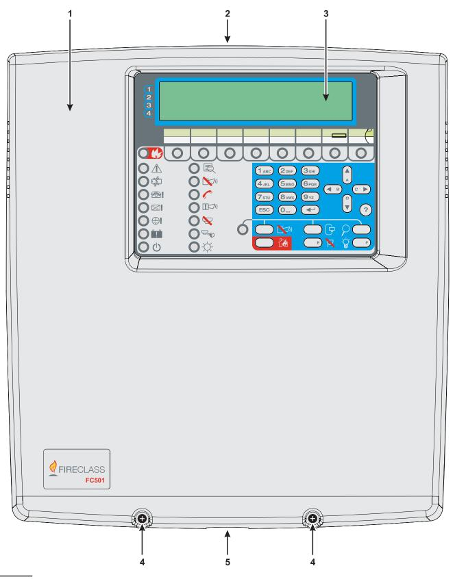
Figure 1 FC501 Parts: external view.
