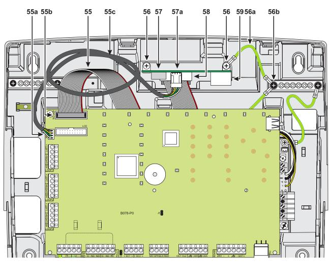
Figure 13 FC501 connection with the FC500IP.
