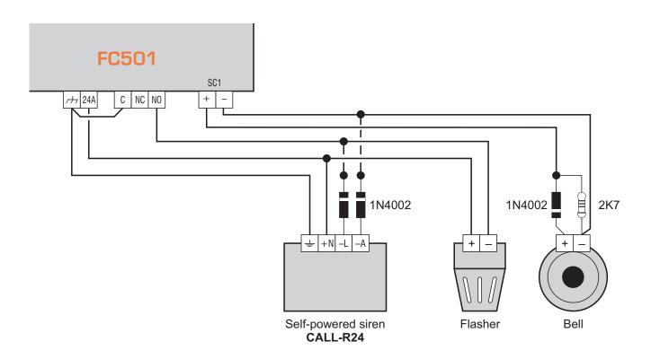
Figure 10 Wiring diagram: NON-silenceable and Silenceable Output connections.
