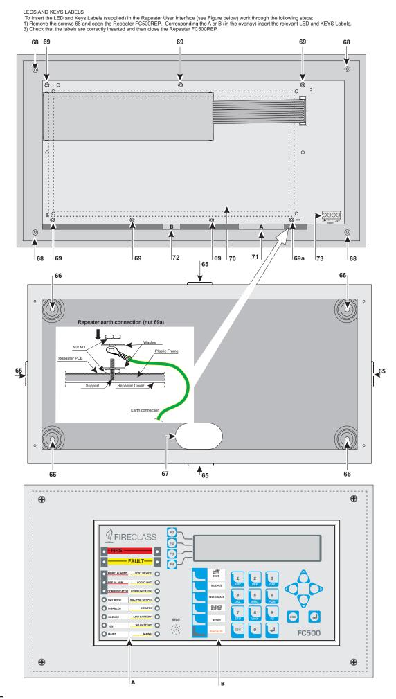
Figure 5 Installation FC500REP Repeater.
