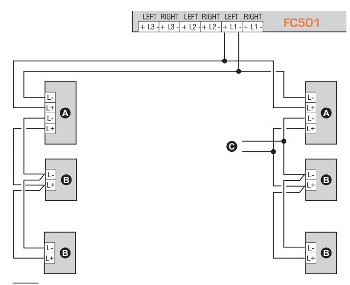
**Figure 6** Wiring diagram of a 2-wire connection, a) Isolators; b) Compatible analogue devices (Fire detector, Input modules, Output modules, Manual callpoints); c) T connection.
