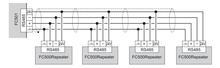
Figure 8 Wiring diagram of four (max) (FC500REP) Repeaters connected to the RS485.
