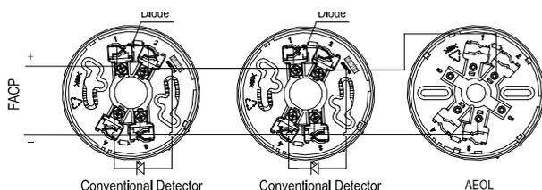
The typical connection of End of Line Resistor
