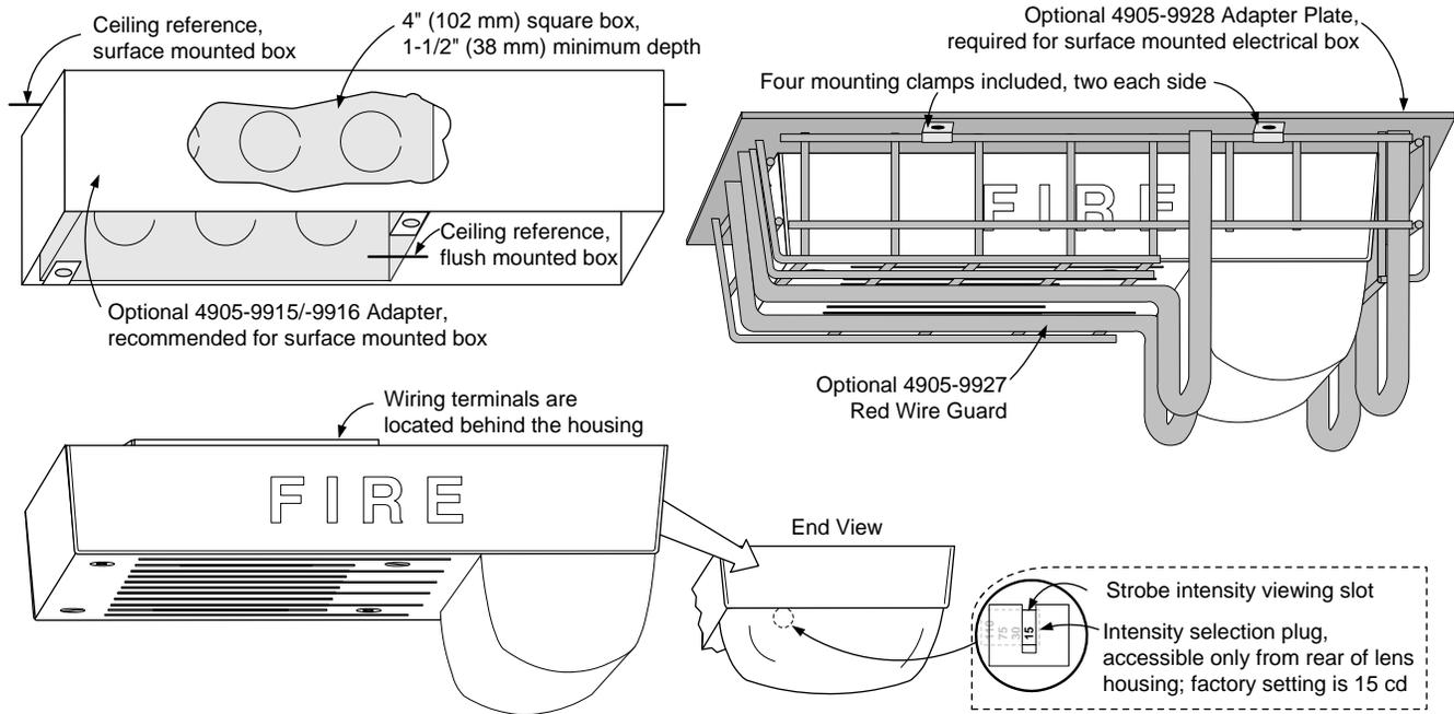
**Wall Mount Installation Reference; Adapter Plate, Guard, and Adapter Skirt**
