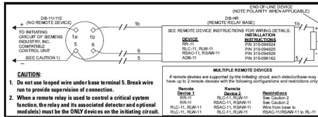
**Note:** The illustration above is typical wiring for Models DB-11 and DB-11E (using Models PE-11, PE-11T, DT-11, OP121, OH121, and HI121 detectors).
