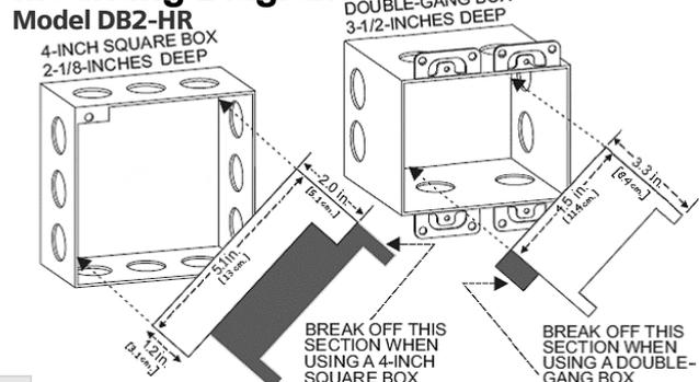
**Notes:** The Module Barrier (shown to the right) must be used when Model DB2-HR relay contacts are connected to non-power-limited circuits. Break apart the barrier to the correct size and shape for either the 4-inch square or double-gang box. Install the barrier diagonally into the back box to create two (2), separate compartments with the back box, in order to separate the wires.
