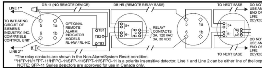
**Note:** The illustration above is typical wiring for Models DB-11 and DB-11E (using Models HFP-11 Series and SFP-11 Series detectors).
