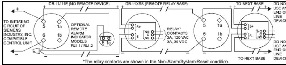
**Note:** The illustration above is typical wiring for Models DB-11 and DB-11E (using Models FP-11, FPT-11, FS-DP, FS-DPT, and FS-DT detectors).
