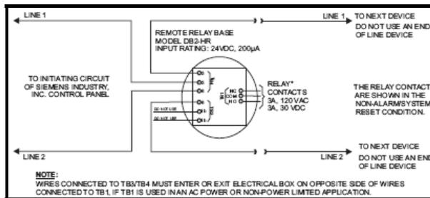
**Note:** The illustration above is typical wiring for Model DB2-HR for polarity-insensitive detectors).
