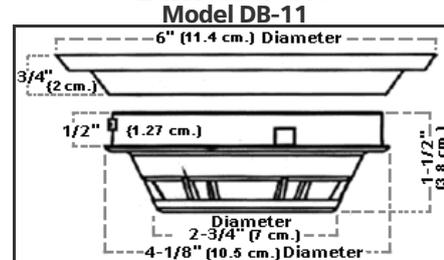
**Note:** Model DB-11E base detector has a diameter dimension of 4.5" (11.4 cm.).
